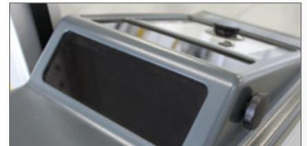
The headlights are aligned via the projection screen that is visible from the side of the vehicle. Border lines printed on the screen are used to compare the actual value with the target value and facilitate alignment. A deflection mirror makes the headlight projection visible from the front of the unit as well.
