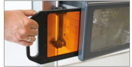
The colour filter should be used in accordance with manufacturer specifications, regardless of the headlight type being tested. The filter makes it easier to determine the cut-off line in the case of pronounced diffusion. The colour filter can be removed by its hand grip to measure the light intensity.
