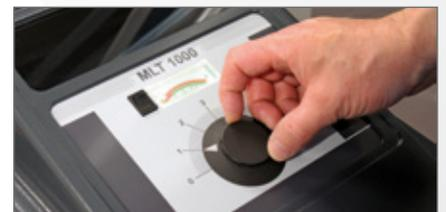
Mechanical height adjustment enables the projection screen to be moved vertically in the housing. The hand wheel fitted with a scale can be used to preset the required inclination angle for the headlight.
