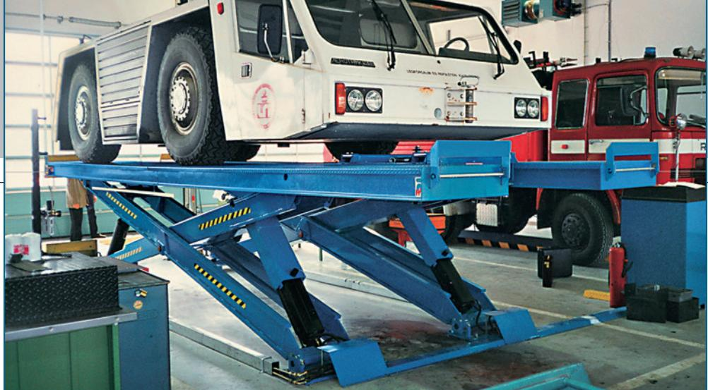
*Because of its big capacity, this lift is to be preferred for particular vehicles such as tank trucks, trucks with crane, fire brigade vehicles and airport tractors. In fact, a capacity of 33T not only enables lifting of heavy loads but also caters for non-favourable load distributions.*
