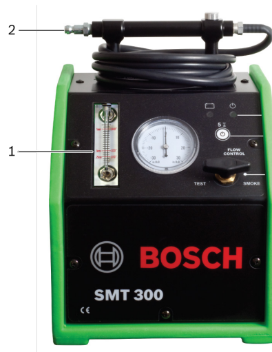
Fig. 8: EVAP test with SMT 300
