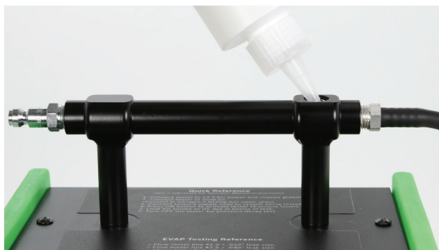
Fig. 5: Filling the UltraTraceUV® smoke solution
